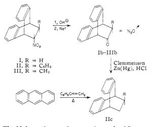
The Nef reaction on the potassium salt of I gave the corresponding ketone Ib in 87% crude yield. This, and its oxime, were identical with the corre-
